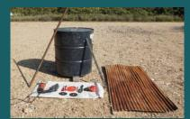
**Tools**: Drill, drill bits, plyers, string, marker **Materials from recycling**: barrel, 2 sheets of roofing metal, 2 m 1" steel box,
